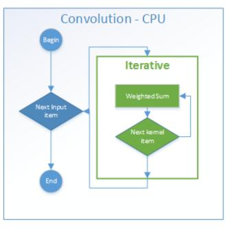
Fig. 5. Flow of sequential filtering algorithm.
