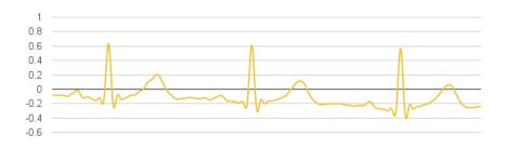
Fig. 8. The ECG signal filtered with a low pass filter of 30Hz.
