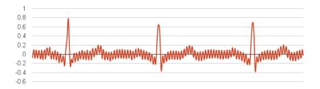
Fig. 9. The ECG signal filtered with a high pass filter of 0.5Hz.
