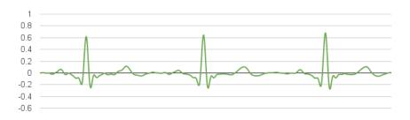
Fig. 10. The ECG signal filtered with a band pass filter between 0.5Hz and 30Hz.
