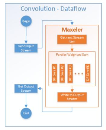
Fig. 6. Parallel Dataflow Computation algorithm.
